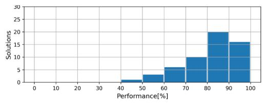
Fig. 5. Thermal error compensation performance of machine learning models
