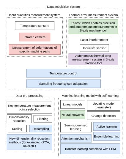
Fig. 6. Graphical representation of this review results. It is showed that, thermal error compensation is developed in three areas (data acquisition, data pre-processing and machine learning model with self-learning). Legend: green – preferred methods, red – very expensive methods, blue – new possibilities of improvement, purple – future challenge
