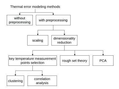
Fig. 4. Division of thermal error modelling methods with regard to data processing
